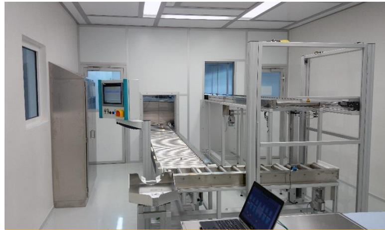
The cleaned parts exit into a cleanroom through an airlock.
